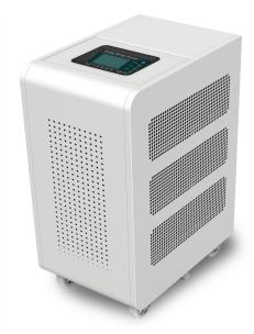
**SUN GB Series** is a single phase multi-function energy storage inverter, combining functions of inverter, On Grid, MPPT Solar charger controller and AC battery charger to offer uninterruptible power support with portable size. Its comprehensive LCD display offers user-configurable and easy-accessible button operation such as battery charging current, AC/Solar charger priority and acceptable input voltage based on different applications.
