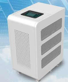
SUN GBT Series is a Three phase multi-function energy storage inverter, combining functions of inverter, On Grid, MPPT Solar charger controller and AC battery charger to offer uninterruptible power support with portable size. Its comprehensive LCD display offers user-configurable and easy-accessible button operation such as battery charging current, AC/Solar charger priority and acceptable input voltage based on different applications.
